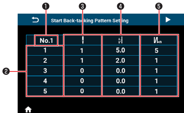
Sewing-start condensation custom setting screen
